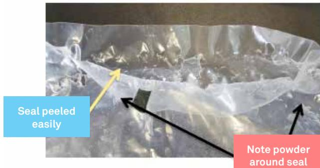
**Figure 5.** Seal failure in many seals due to peeling, particularly where powder was observed.
