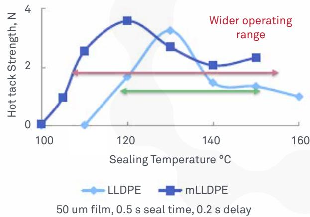
**Figure 3. Hot tack strength test of LLDPE and mLLDPE polymers**
