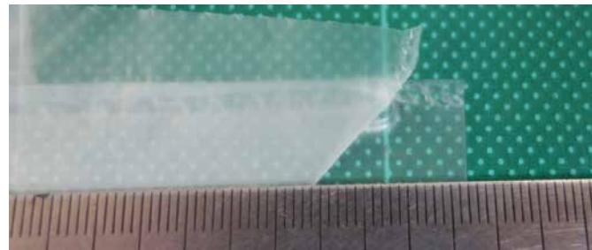
**Figure 7.** Seal failure of a HDPE bag
