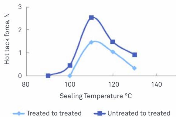
**Figure 4. Effects of corona treatment on sealing. Attempting to seal two treated surfaces to each other results in lower hot tack strength and a narrow sealing temperature range.**
